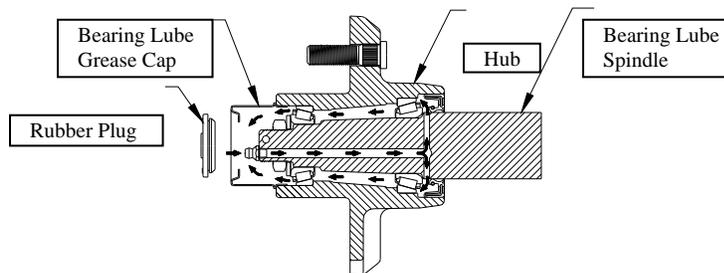
For units that are not equipped with the Sure Lube or Bearing Lube greasing system, the bearings must be packed with grease (by hand) prior to assembly, or at intervals as outlined in the maintenance schedule on page 28 of this manual.
