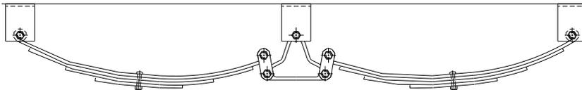
Double eye leaf springs have eyes formed in each end of the spring and are attached to the trailer as follows:
