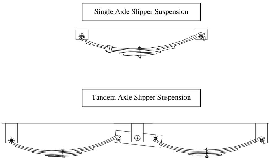
Slipper springs have an eye formed in one end only with the other end formed into a reverse curve. The attachment of these springs is as follows:
