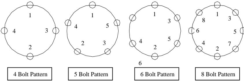
1. Start all bolts or nuts by hand to prevent cross threading.
